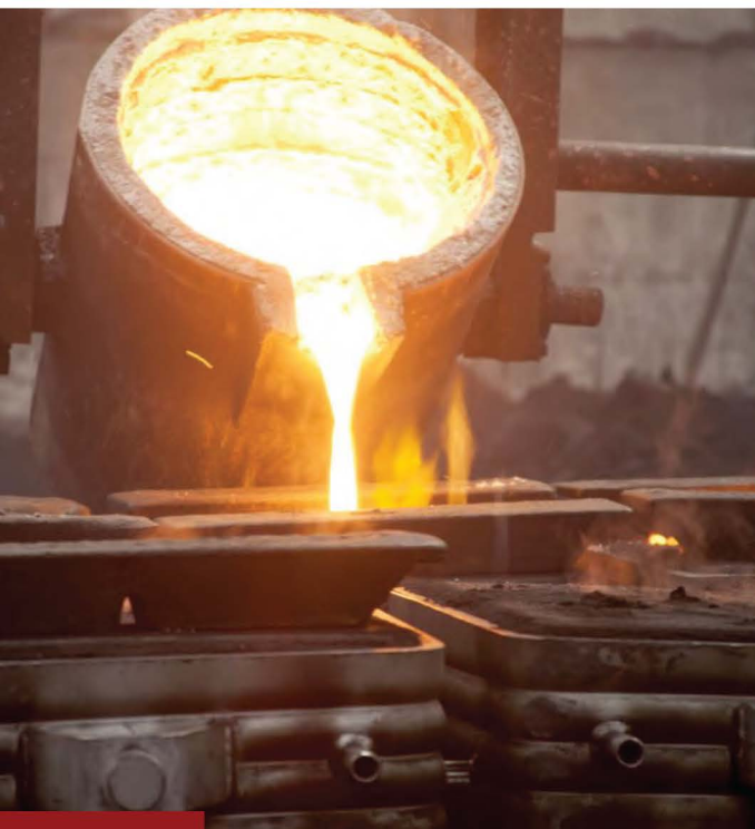
Casting of metal components
