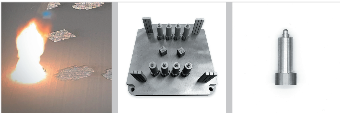
Left: Area Printing melts powder to form one of the steel core pins for UAT's ICC clamp. Center is 8 core pins (4 in the front, 4 in the back) with tensile bars and test cubes also on the build plate. Right showcases the finished part, which is a single core pin, printed in SS 316.
